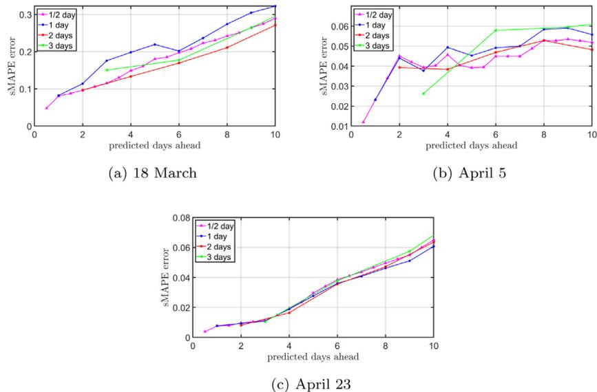
**Fig. G.8.** (Method B: First smooth, then remove.) The NIPA prediction accuracy for the situation in the Netherlands for varying time steps  $\Delta t$ . The subplots show the forecast for (a) March 18, (b) April 5, and (c) April 23. For the time step  $\Delta t = 2$  days and  $\Delta t = 3$  days, the data is first smoothed and then removed.
